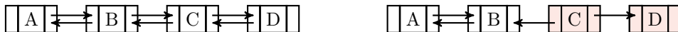
Figure 1.4: Naïve removal for doubly linked Lists. Deleting all references pointing to C deletes the node, but it also separates nodes A and B from node D.
