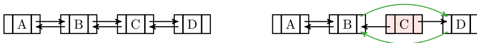
Figure 1.5: Correct removal for doubly linked Lists. To avoid gaps in the chain, nodes B and D must be linked together.
