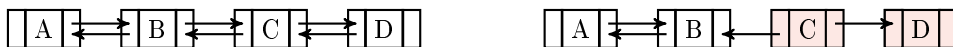
Figure 1.4: Naïve removal for doubly linked Lists. Deleting all references pointing to C deletes the node, but it also separates nodes A and B from node D.
